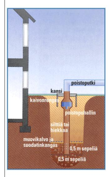
Radon well, from bottom: coarse crushed material, plastic sheet and filter cloth, fine sand or silt, fan, well deck and outlet piping
